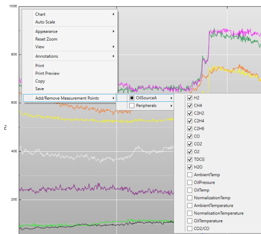
Figure 4-9: Remove measurements from the trend chart
